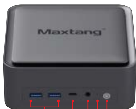
2x USB3.2 Audio Power Button CLR_CMOS USB-C(USB3.2_10Gb)
