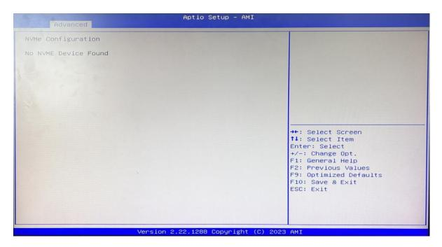
The capacity and model of the SSD will be displayed under the option after the NVMe protocol SSD has been installed.
