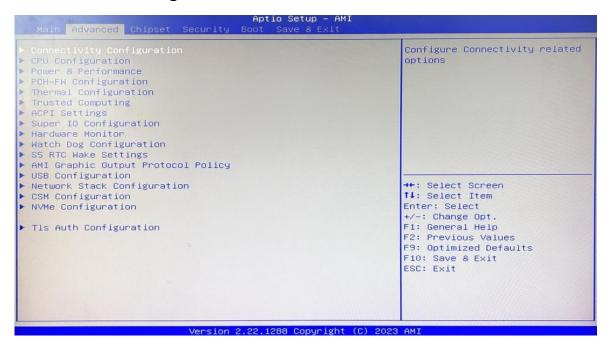
Select any of the items in the left frame of the screen. The advanced sections allow you to configure, improve and set up system features according to the preference of the CPU Configuration. All Advanced BIOS Setup options are described as follows.
